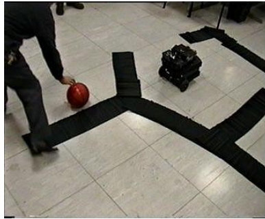
Fig. 6. ART Pioneer robot follows the ball while avoiding black obstacles
