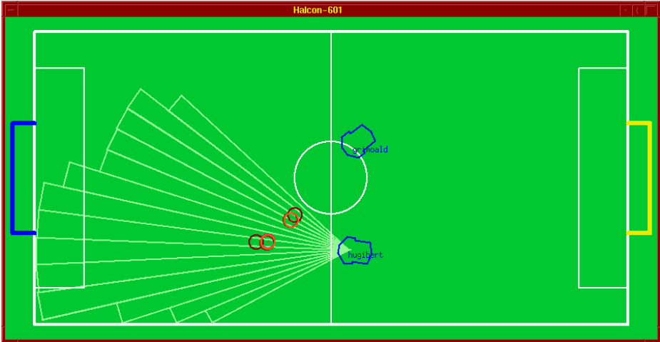
Fig. 6. The RoboCup monitor visualizes the actual positions of robots, ball hypotheses and free motion spaces.
